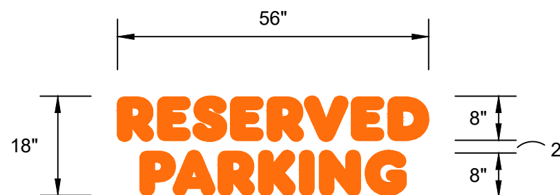
"RESERVED PARKING" SHOULD BE PAINTED ON THE TOP OF THE PARKING STALL (CURB SIDE) SCALE : N.T.S.
